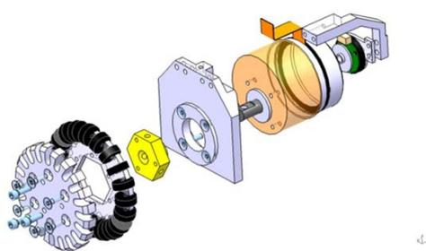
**Fig.1** Exploded view of the driving system
