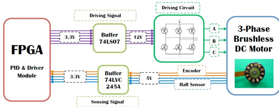
Fig.6 Motor drive system
