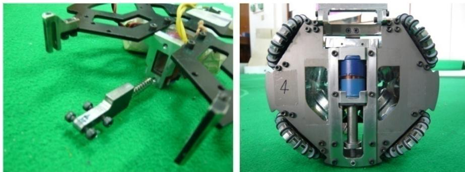
**Fig.3** Chip-kick solenoid rod (left) and bottom view of robot (right)
