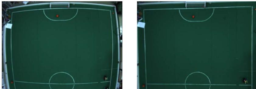
**Fig.8** Distorted image (left) and undistorted image (right)
