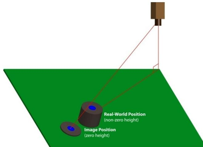
**Fig.10** Comparison between zero and non-zero robot's height
