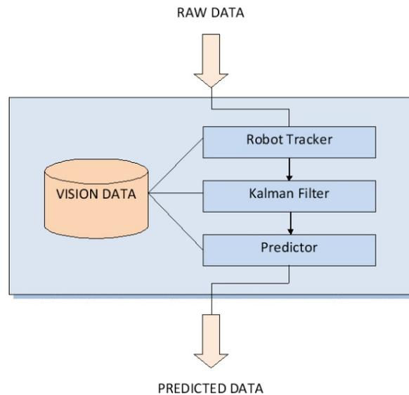
Fig.11 Vision filtering
