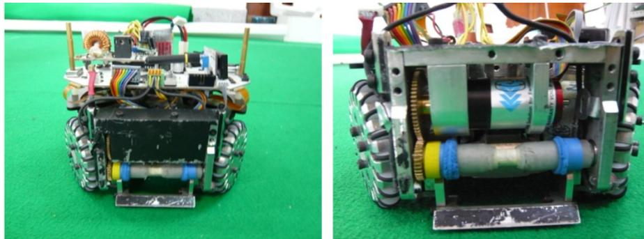
Fig.4 Front view of the robot (left) and inner mechanism of dribbler (right)
