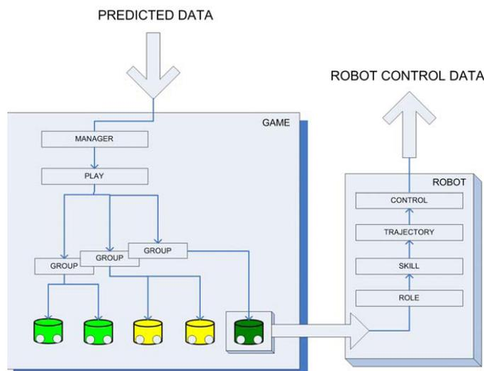
**Fig.12** AI's layer architecture
