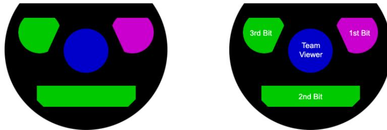
**Fig.9** Robot's head pattern (left) and illustration of colors representing robot number (right)
