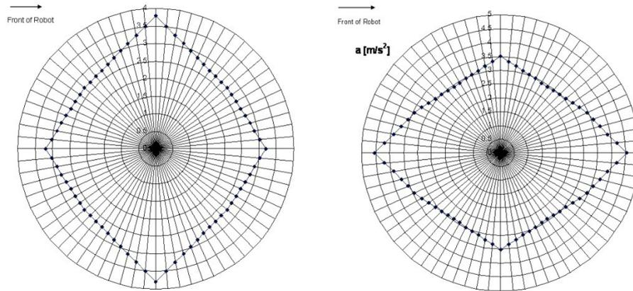
**Fig.2** Velocity profile of the robot (left) and acceleration profile of the robot (right)
